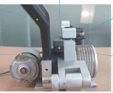
Screw to adjust the space between friciton parts
